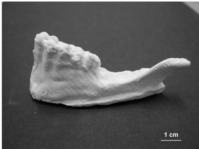
Fig. 12. Human jaw-bone made of hydroxyapatite by freeze casting in ice moulds.
